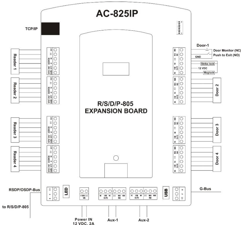
AUX1 and AUX 2 are additional auxiliary inputs and auxiliary outputs. Refer to Chapter 2 for maximum power ratings and further information.
