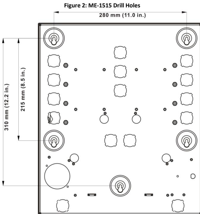
2. Insert masonry anchors into the drilled holes.
