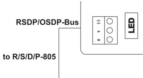
Any subsequent expansions are connected to each other using the RSDP bus located the bottom center of the expansion (Figure 19).
