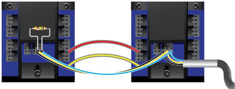
If multi-pair twisted pair cable is used, one pair shall be used for A+ and B- signals (blue and white/blue) and one pair for GND (orange + white/orange). Unused wires should be terminated with 100  $\Omega$  resistors to ground at both ends of the cable.
