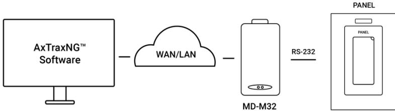
The maximum distance from the Ethernet port of the panel to the LAN/WAN connection is 100 m (330 ft).
