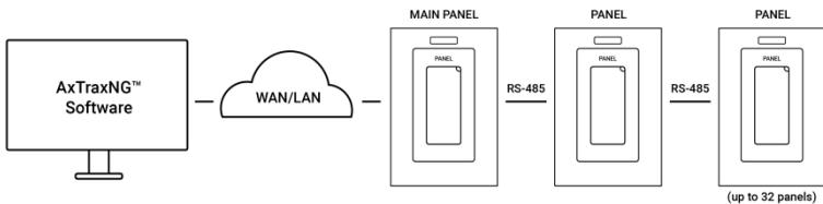
To connect to a TCP/IP network using AC-425 non-IP models, add Rosslare's MD-N32 TCP/IP to RS-232 gateway converter.
