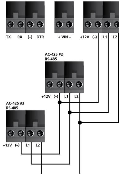
This can increase the maximum distance from the PC to the last panel in the chain to 4,000 ft (1,219.2 m).
