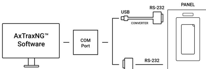
The distance between the computer and the access control panel must be no more than 150 feet (50 meters).
