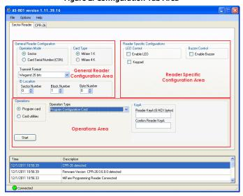
Figure 2: Configuration Tab Area
