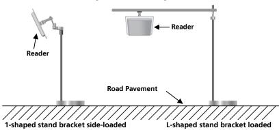
Each installation method is selected based on application requirements and actual location. The user can use the provided template to install AY-U910 reader in more convenient and easier way, but the read distance is a little short; the situation becomes opposite if using the latter.
