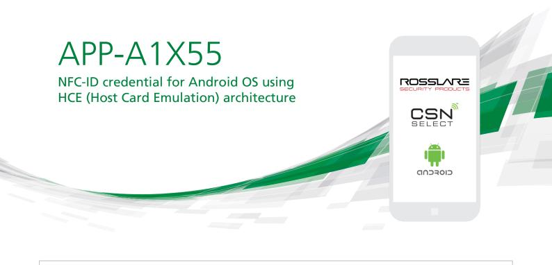
Rosslare created the APP-A1X55 app for adding the HCE service to Android devices, supporting NFC to be used with a variety of Rosslare's physical access control readers that support NFC technology. The app, which runs in the background, provides an NFC unique ID (UID) based on the device fixed parameters.
