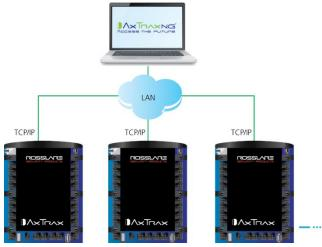
The maximum distance from the Ethernet port of the panel to the LAN connection is 99.97 m (328 ft).
