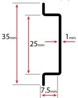
Figure 10: DIN Rail Dimensions (Top View)
