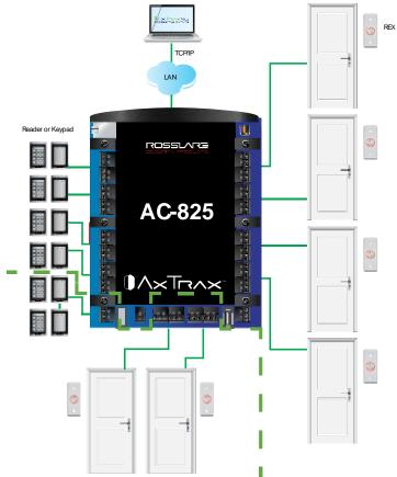
Figure 1: Sample AC-825IP Configuration
