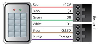
Figure 22: Reader Wiring – OSDP
