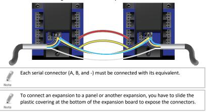
The RS-485 bus must be terminated at both ends of the cable with a 100-120  $\Omega$  resistor (Figure 20).
