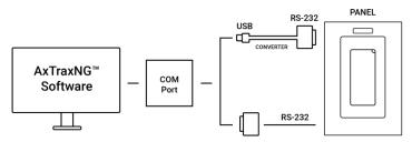
The distance between the computer and the access control panel must be no more than 150 feet (50 meters).
