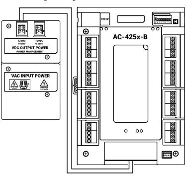
Figure 6: Wiring Between PM-10 and AC-425x-B
