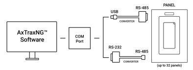
Use the RS-485 interface for situations where there are multiple controllers connected. The serial port used to control the access control panel is assigned within the AxTraxNG/AxTraxPro Access Control Management Software.
