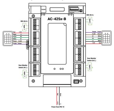
Figure 7: AC-425x-B Wiring Communications
