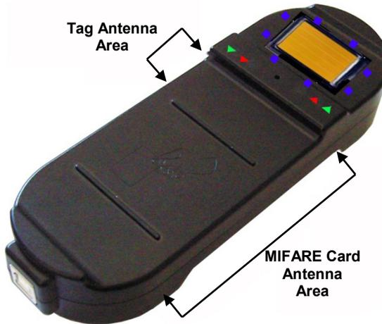
The CP-R26 Programmer configures four card or tags types. The four card types are:
