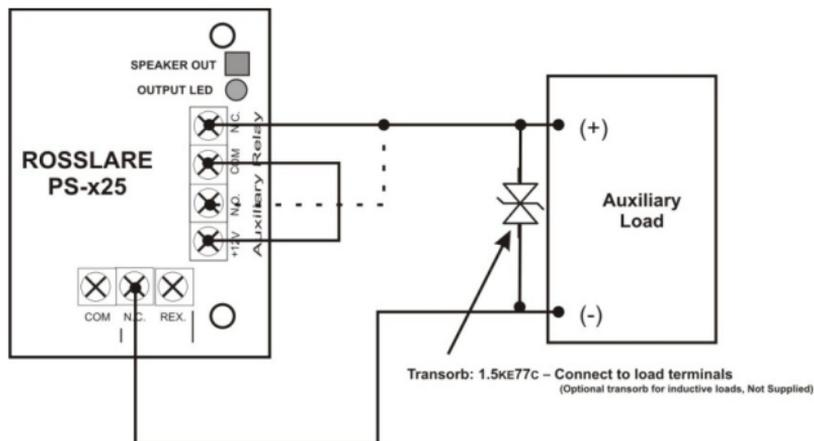
Figure 6 shows the auxiliary output connection using the external power.
