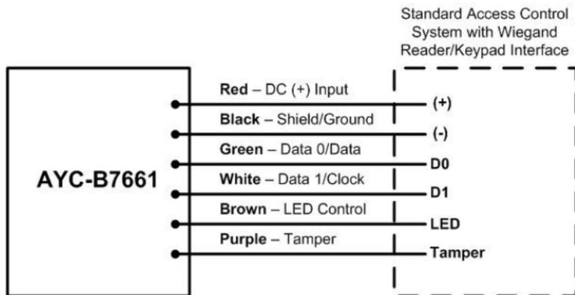
The AYC-B7661 unit is connected with an 8-wire, 46-cm (18") cable.
