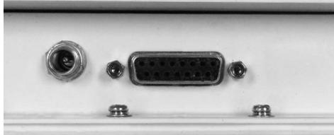
The unit operation voltage is 9–12 VDC, by an independent power supply connected to the 2-pin power interface.
