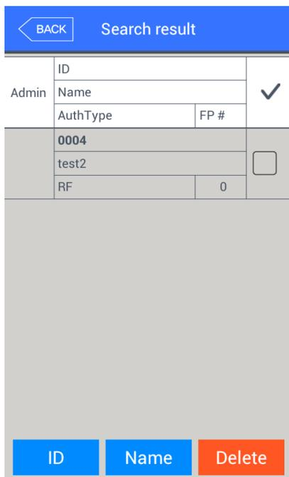
► **[Name]:** Press the button and input user name to display registered user list with the name in which input character string is included. Press **[BACK]** button in this screen to move to '3.3. User management' menu.
