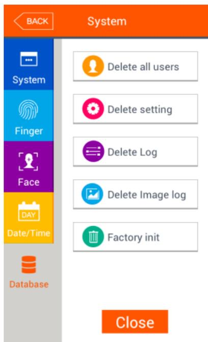
To delete all users, press **[Delete all users]** button. To reset the setting value, press **[Delete setting]** button. To reset authentication record, press **[Delete Log]** button. To delete only image log, press **[Delete image log]** button. To delete the whole data to make the device to factory setting status, press **[Factory Init]** button.
