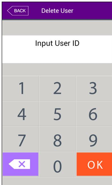
Input user ID to be deleted and press **[OK]** button. Press **[BACK]** button to cancel and move out.
