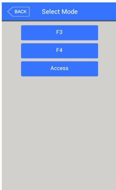
Press desired access mode button in access mode selection screen in the left to close selection screen and to convert mode in the main screen into the relevant mode.
