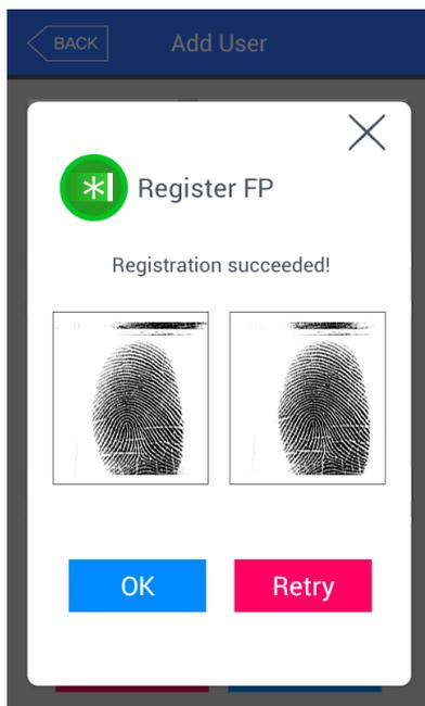
④ Message on the left will be displayed when input is completed. Press [OK] button to complete registration and move to the upper menu.
