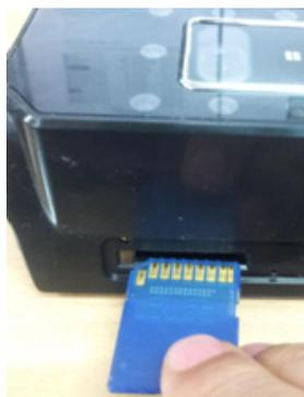
This function is to backup data of the terminal using **[EXPORT]**. Data backed up by **[IMPORT]** can be copied back to the terminal.
